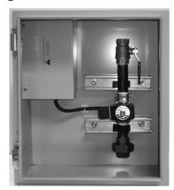
The *ISIMET* Laboratory Service Panel operates as a single output controller incorporating either a solenoid valve assembly or electrical contacts along with the digital switching mechanism within a single enclosure. An internal junction box houses the 120-vac line voltage along with transformer and circuit board.
